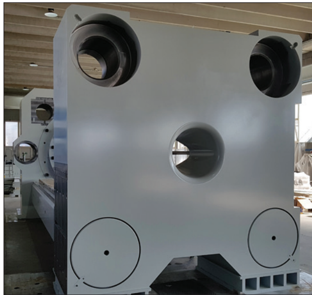
Figure 2. Front platen for one of the 50 MN presses.
